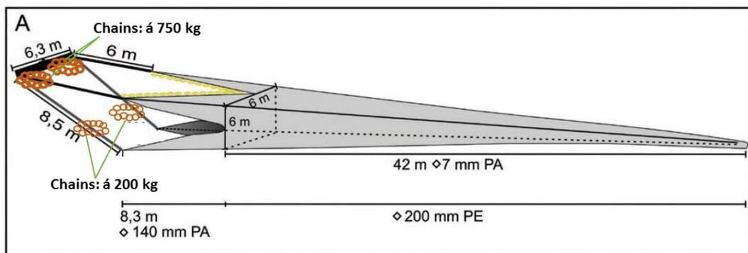
**Fig. 5.** Schematic drawing of the trawl dimensions and rigging.
