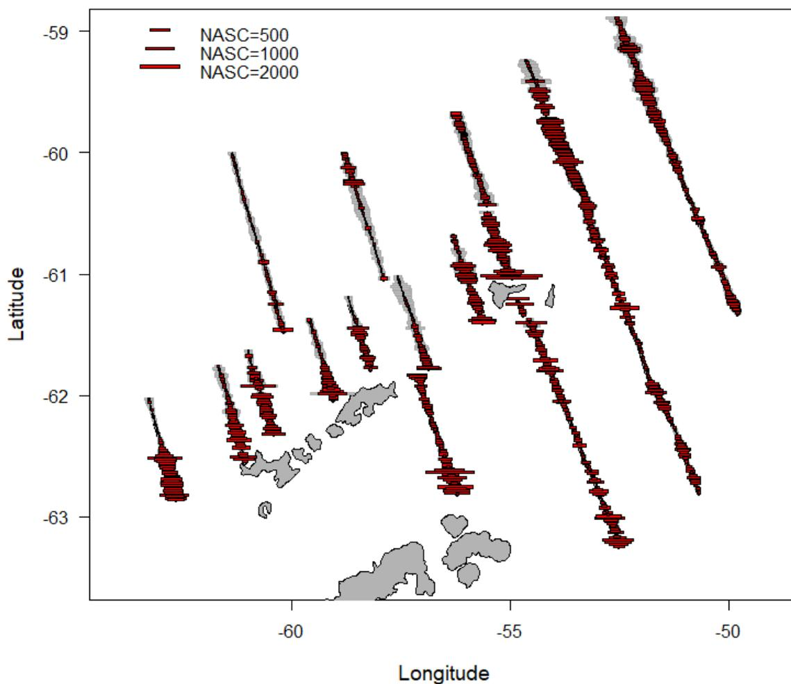
**Fig. 11 a)** Distribution of acoustic backscatter (Nautical Area Scattering Coefficient; NASC;  $\text{m}^2\text{nmi}^{-2}$ ) integrated over 1 nautical mile, allocated to krill (red) and other targets (grey). The NASC-values are square root transformed.
