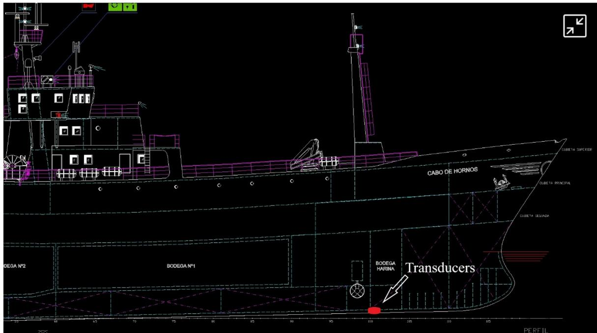
**Fig. 3.** Positioning of the transducers on board the ‘Cabo de Hornos’.
