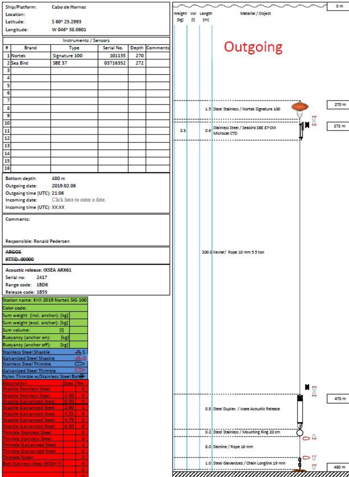
Fig. AIV\_3) Data sheet for deployment of Nortek Signature 100 echosounder and current profiler mounted together with Seabird CTD.
