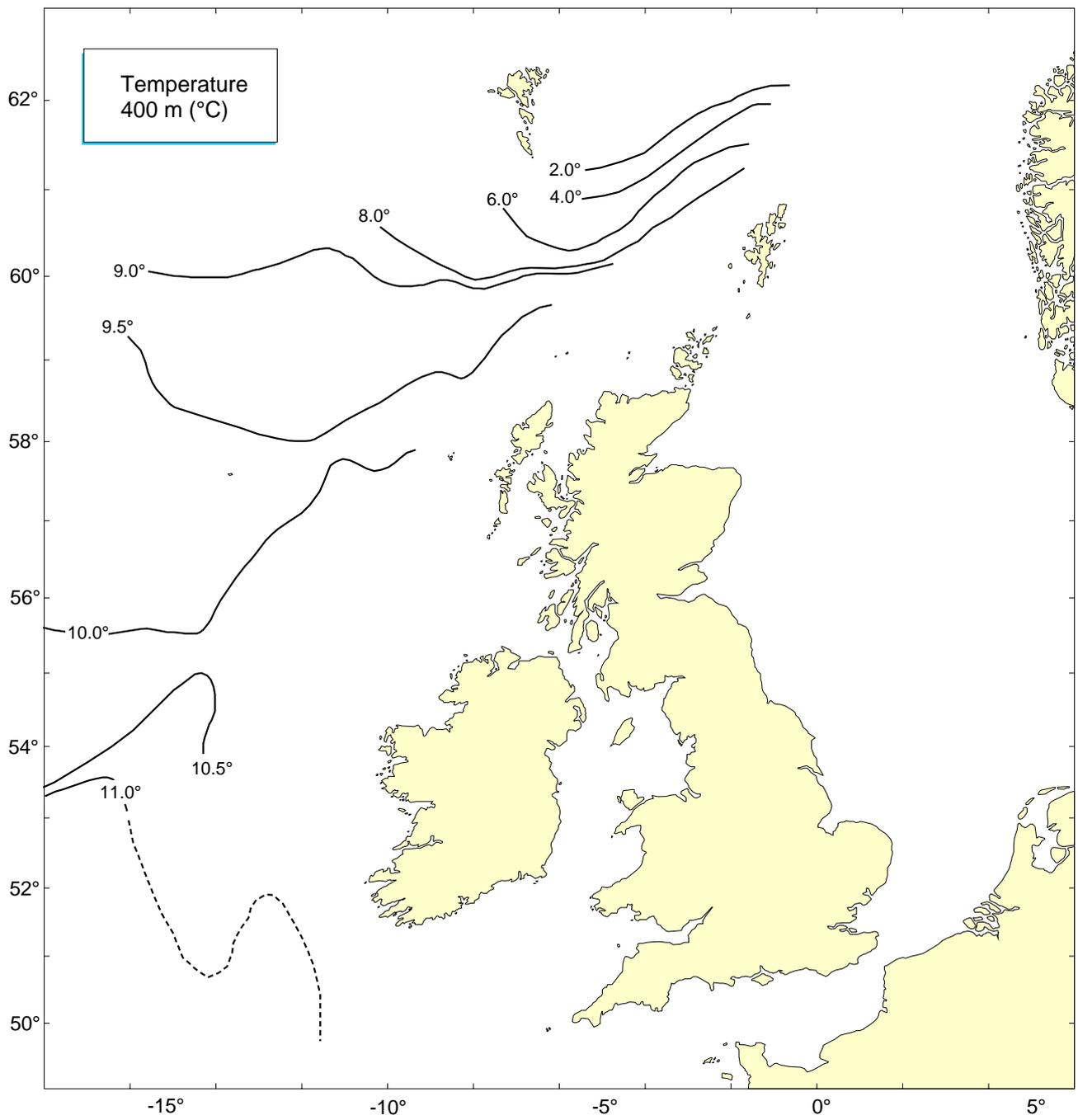
Figure 9. Horizontal temperature distribution, °C, at 400m depth
