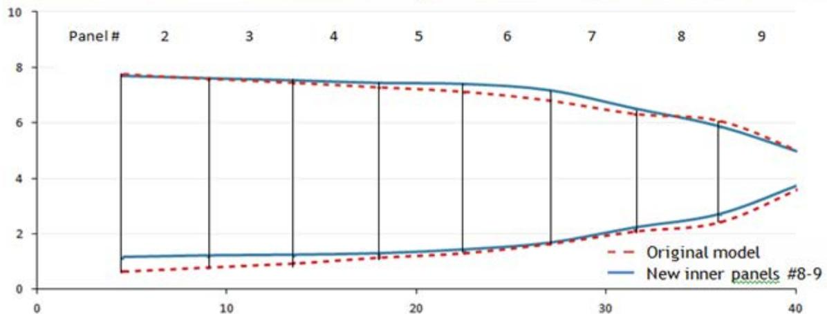
**Figure 3.** Change in the shape of the trawl. Before (upper left) and after (upper right) the inner panels # 8-9 were altered, and the cross-section view of inner panels #2-9 (lower; plotted from measurements made from rail-camera rig outside the tank). The inner panels # 2-9 are indicated at the top. The red dashed line is the original shape (test 3) and the solid blue line is with the altered inner panels # 8-9 (test 6).
