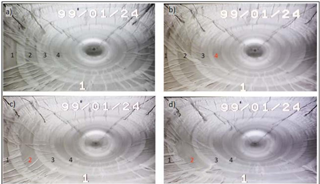
**Figure 2:** View of inner panels, looking back to the codend, during four of the flume tank tests. a) the original model at 6m wing spread, b) the original model at 12m wing spread, c) a 20% reduction in inner panel #2 circumference and d) a 30% reduction in inner panel #2 circumference. The inner panels #1-4 are labeled in each picture. Red numbers indicate the panels with an improvement in the trawl performance.
