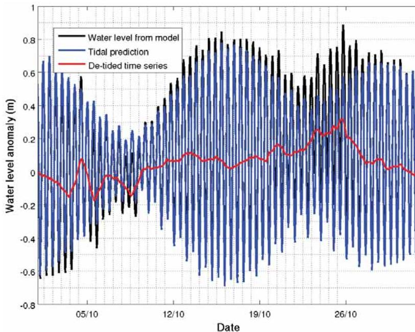
**Figure 10.** Time series of modelled sea level (black line), and its tidal (blue line) and detided (red line) prediction from October 2008 at the Sognesjøen location from the Hordaland-simulation. The horizontal axis denotes time and the vertical axis denotes sea level height with respect to a mean level.
