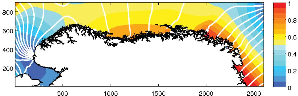
**Figure 5.** Co-tidal range (colors) and co-tidal lines (white lines) interpolated from the TPXO database to the entire NorKyst-800 grid. The spacing of the co-tidal lines is one hour and the equidistance of the co-tidal range is 0.1m.
