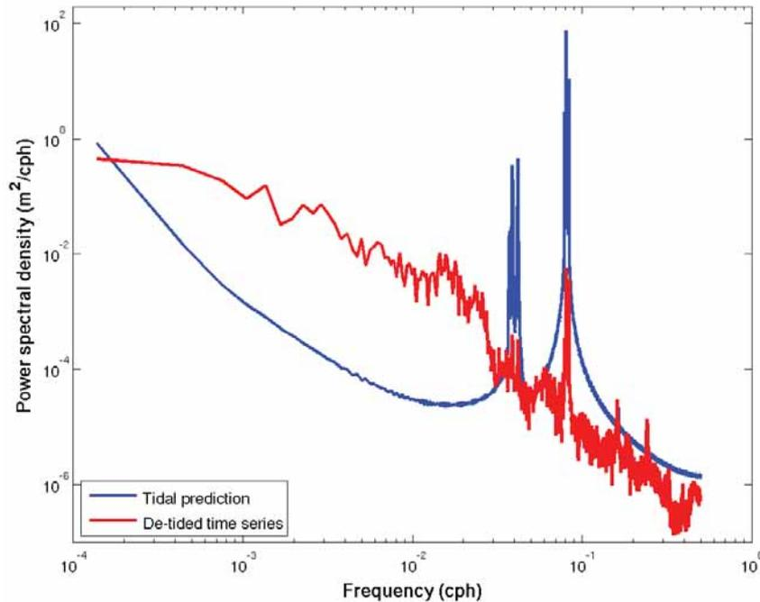
**Figure 11.** Power spectral densities of the tidal predictions (blue line) and the detided time series (red line) at the Sognesjøen location from the Hordaland-simulation for the period January 2008 to May 2010. The horizontal and vertical axes denote frequency (in cycles per hour) and power spectral ( $\text{m}^2/\text{cph}$ ), respectively.
