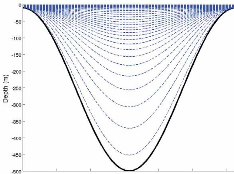
**Figure 8.** Example of the vertical distribution of the s-levels in ROMS when applying the default values of  $\theta_s$  (8.0),  $\theta_b$  (0.1), Tcline (10m) and N (35), where the latter is number of vertical levels. The black line denotes the bottom, and the dashed blue lines denote the s-levels (of rho-surfaces). Depth is given by the vertical axis in m.
