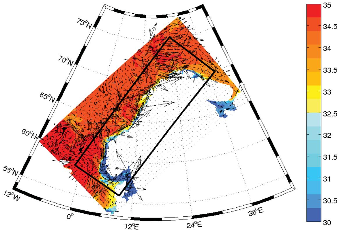
**Figure 4.** Example map from the ROMS hindcast model of the Nordic-4km domain showing SSS (colors) and surface currents. Every 12<sup>th</sup> current arrow is shown, i.e., internal spacing between vectors is approximately 50km. The entire NorKyst-800 domain is indicated by the black square.
