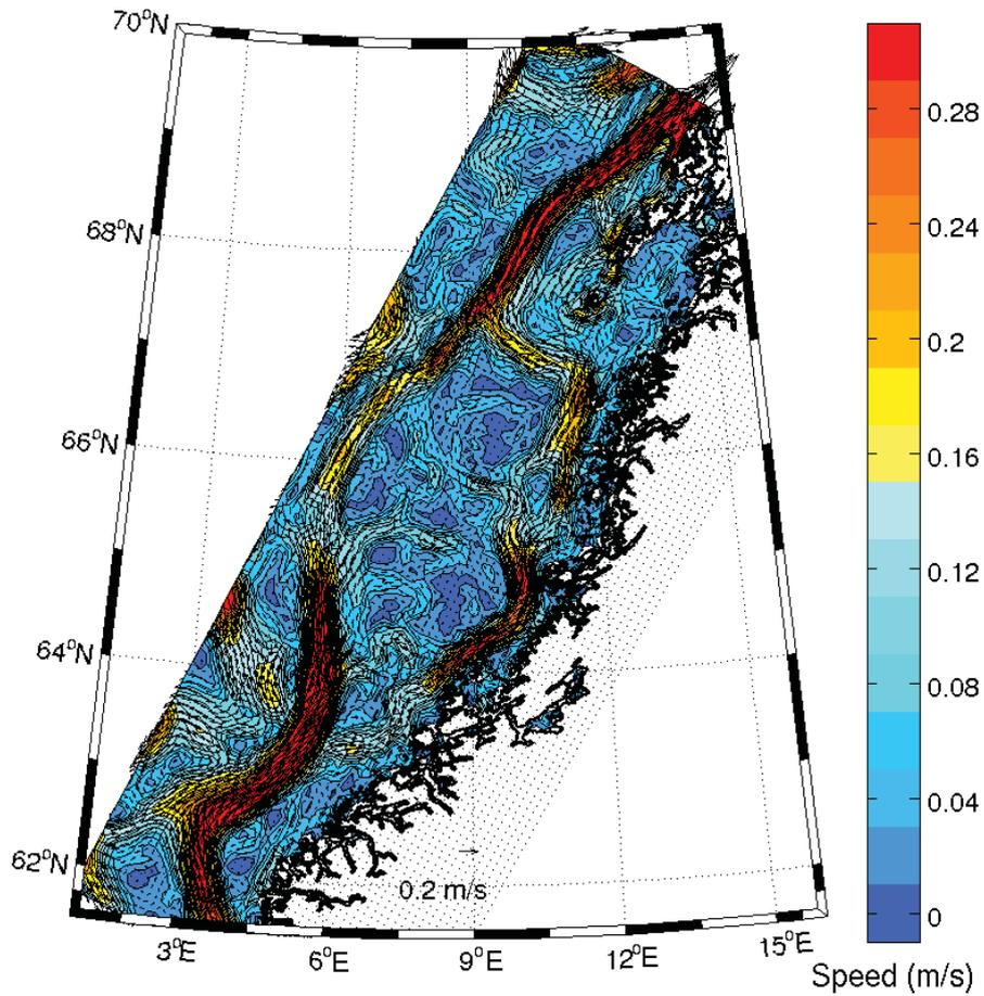
**Figure 12.** Sea surface currents from the Møre-to-Lofoten model realizations averaged over its simulation period (exclusive spin up), see Table 2 for details. The color scale denotes current speed and line interval is 0.05 m/s. The magnitude of the arrows refers to the arrow at the bottom. Every 10<sup>th</sup> arrow is shown, i.e., the internal distance is approx. 8 km.
