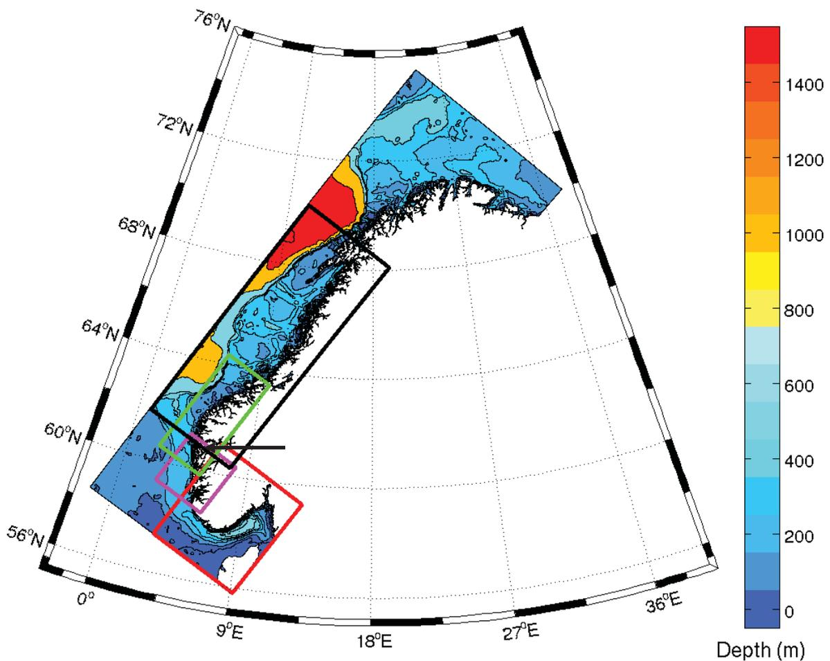
**Figure 9.** Bathymetric chart of the entire NorKyst-800 grid showing frames from the four simulation experiments presented in this report. The red square denote the Skagerrak-run, the magenta square covers the Hordaland coast, the green square the Sogn and Møre coast and the black square covers the shore from Møre to Lofoten. The arrow indicates the position of the Sognesjøen-location.
