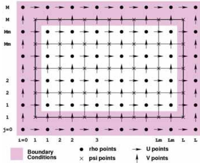
**Figure 7.** Horizontal variable placement on a ROMS grid showing the additional boundary zone (colored in pink for  $i=0$  and  $i=L$  and for  $j=0$  and  $j=M$ ) along the interior grid points denoted by  $1:L_m$  and  $1:M_m$ . The schematic grid structure is downloaded from the <http://myroms.org> web site.
