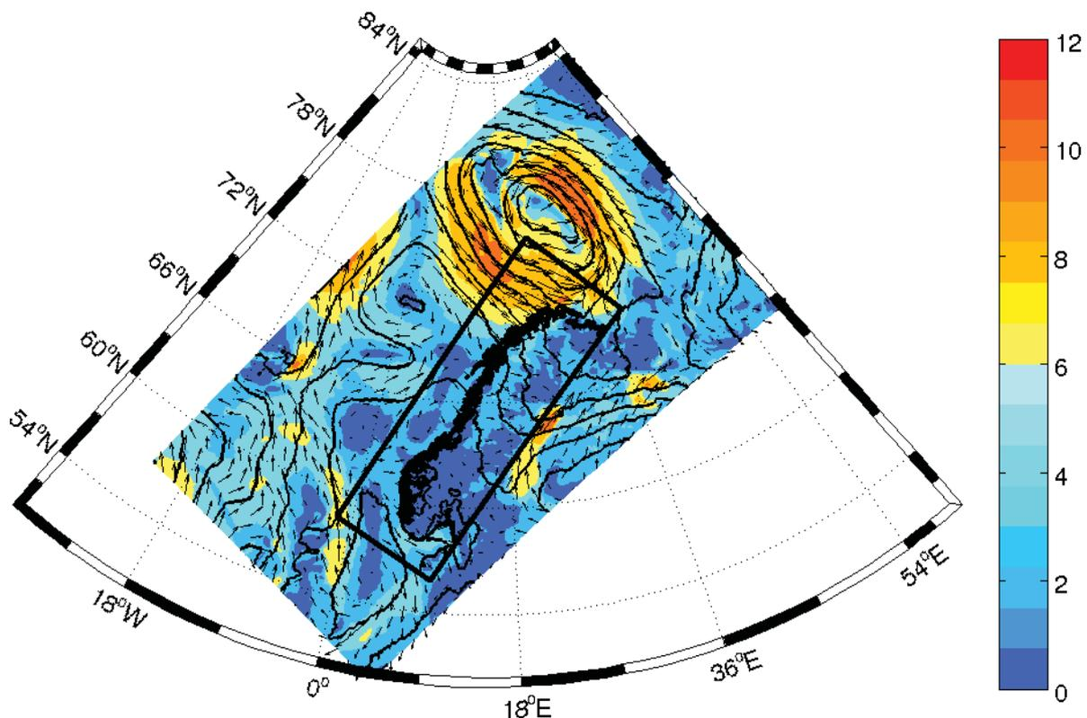
**Figure 2.** Example map from the Hirlam hindcast database showing mean sea level pressure (black lines), wind speed (colors) and wind vectors. Every 10<sup>th</sup> wind arrow is shown, i.e., internal spacing between vectors is approximately 100km. The entire NorKyst-800 domain is indicated by the black square.
